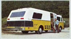
The FMC 2900R is built over a custom chassis, integrating body and frame into a single unit. You're sheathed in a steel beam lower frame and surrounded by an aluminum upper cage.
