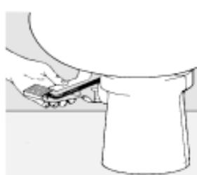
3. Slide pedal cover onto foot pedal rod.
