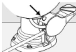
2. Pull on bottom of cover to remove it. Cover snaps back into place.
