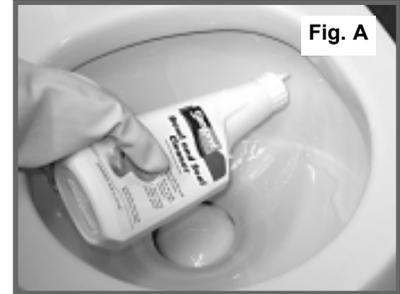
**SEAL CLEANING:** After an extended time, mineral deposits from hard water can build up under the edge of the rubber bowl seal, resulting in a slow leakdown of water from the bowl. To prevent this mineral build-up, periodically clean under the bowl seal with SeaLand Bowl and Seal Cleaner (Fig. B).
